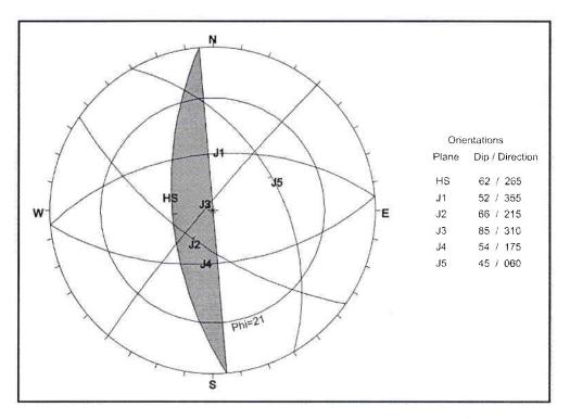
Figure 9: Slope stability analysis at the right bank of weir axis area.
