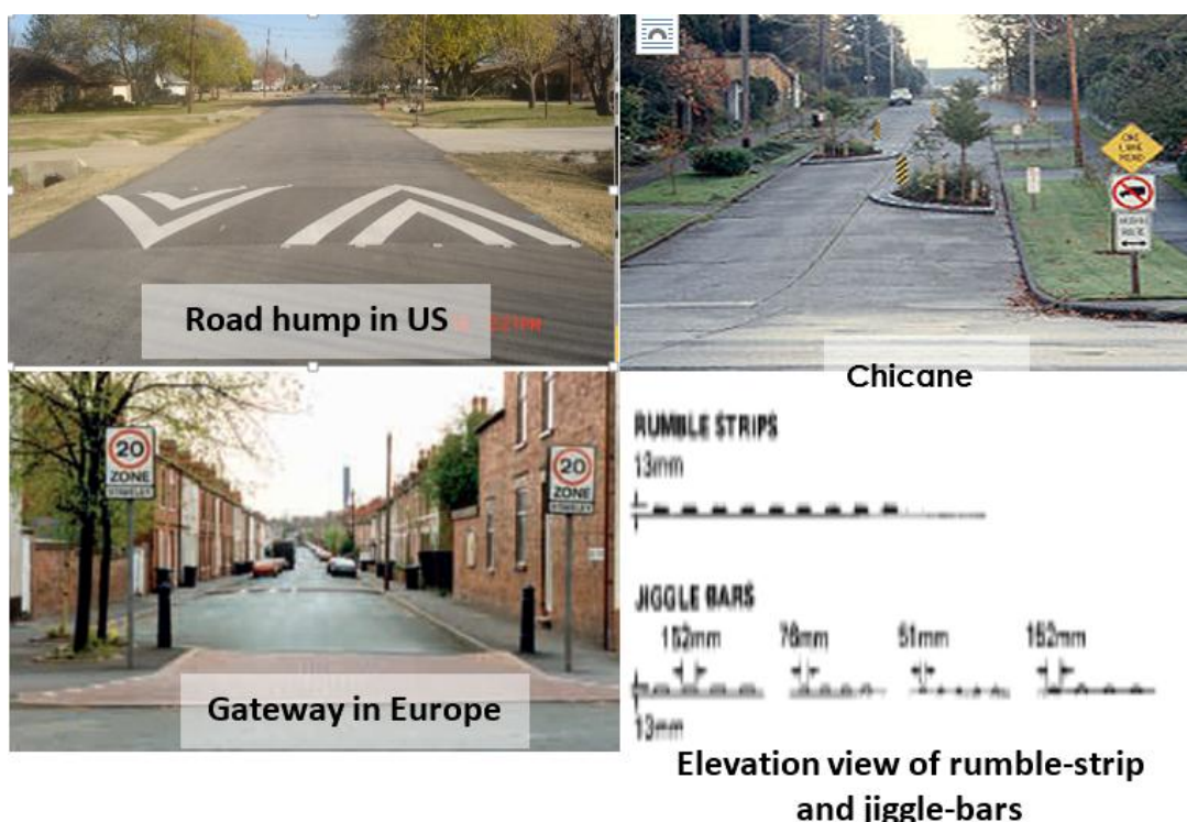
Figure 4.1 Example of Traffic Calming Measures
