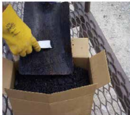
Figure 6.2 Sampling from a Truck Scraping Sample Off Shovel into Sample Box
