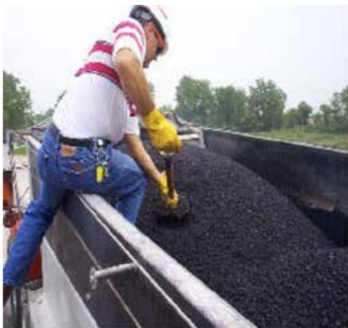
Figure 6.2 Sampling from a Truck Scraping Sample Off Shovel into Sample Box
