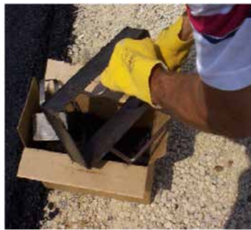
Figure 6.1 Template Placed in Asphalt Mat Cleaning Asphalt Off Template into Sample Container
