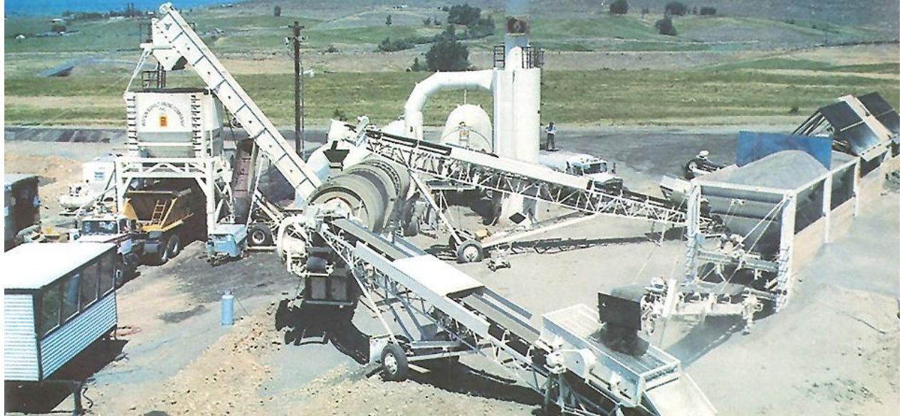
Figure 4.4 A typical parallel-flow drum-mix plant
