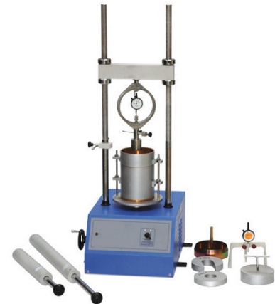
Fig.5.1 Lab-CBR Test Setup
