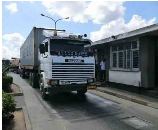
Figure 2.2 Axle Unit Weighbridge
