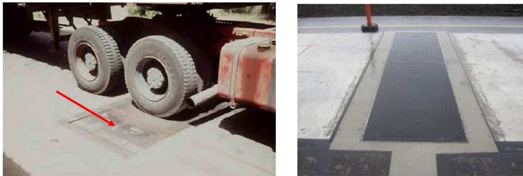
Figure 2.1 Single Axle Weighbridge
