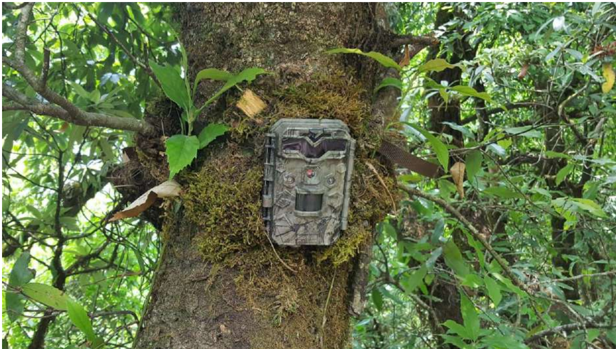
A typical camera trap station setup - camera traps were placed in optimum locations within grids, and secured to trees with chains and padlocks after which they were camouflaged to blend in with the environment to minimise detection/disturbance.
