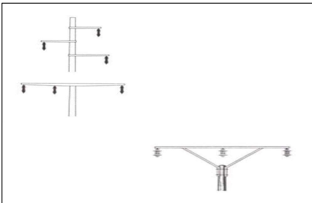
**Figure 6-1: Power poles with suspended insulators**
