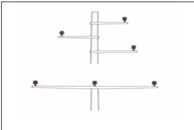
**Figure 6-4: Power poles constructed on pre-stressed concrete or metal with upright insulators rank as the most dangerous of all types**
