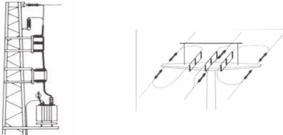
**Figure 6-3: Suggested position of transformer (left image) and an extra insulated perch above the wires (right image)**
