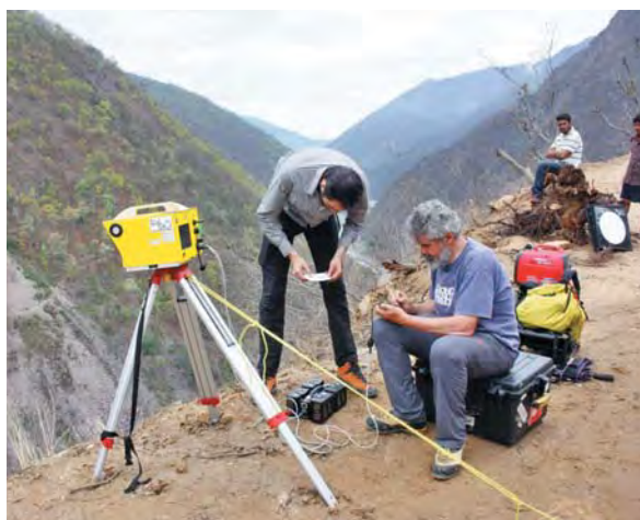
Terrestrial Laser Scanner Survey at Dam Site
