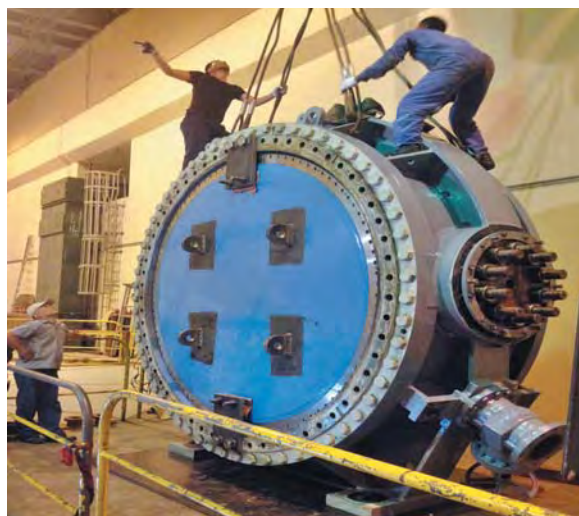
Modified MIV Shifting for Assembly
