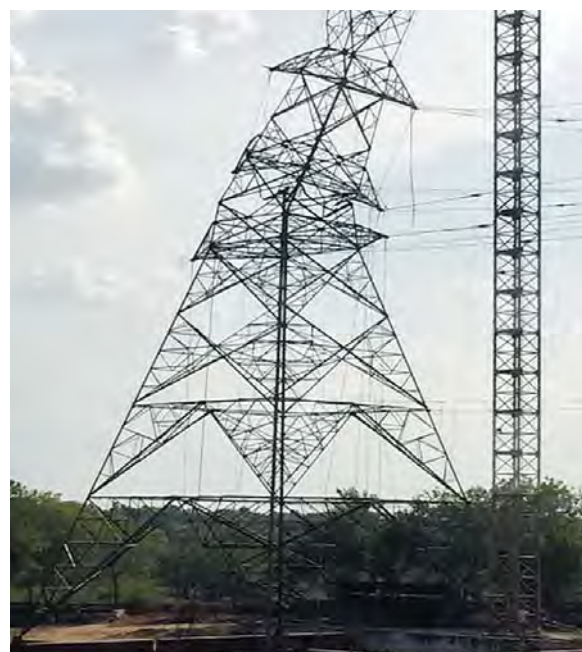
Koshi Corridor Twin Moose DB(t) Tower destruction test at KPTL's Test bed, Gujarat, India
