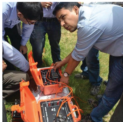
Final inspection and test of New WDJ-4 Digital Resistivity / IP model ERT machine.
