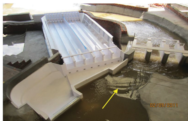
Physical Model of the Kaligandaki A Project
