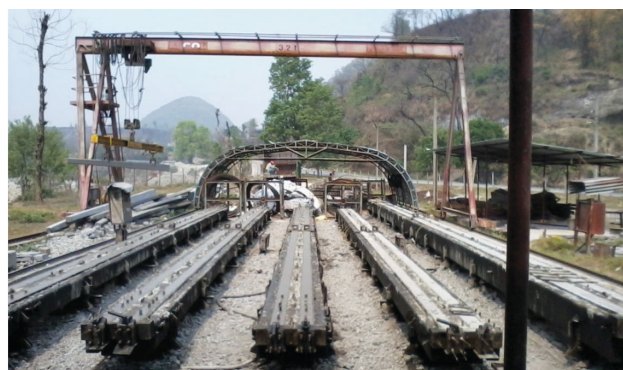
Existing Mould for PSC pole production
