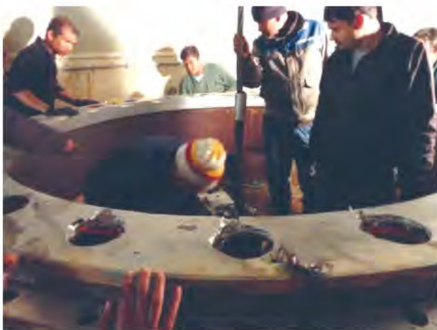
Highly Eroded Bottom Facing Plate due to Silt
