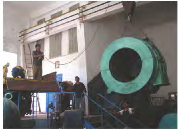
Lifting of Stator during Overhauling
