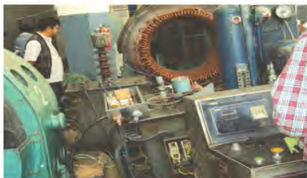
High Voltage Test carried out in newly installed Stator of Unit No. 2
