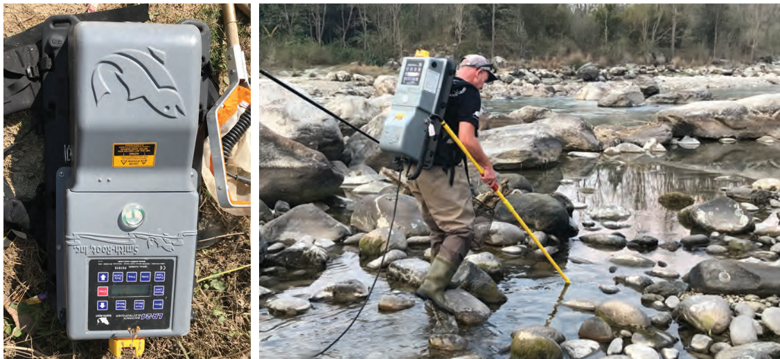
Figure 2.5 Backpack Electrofisher and its use in the Rocky Streams of the Trishuli River Basin
