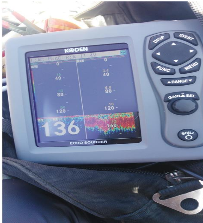
Highest Depth of the Phoksundo Lake Observed by Echo Sounder during the Bathymetric Survey
