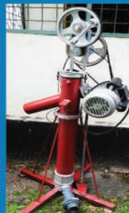
Motorized gulper Capacity: 90 liters/minute
