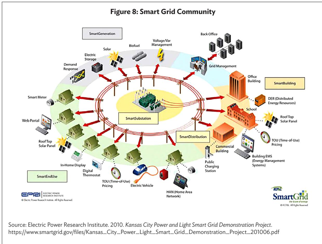
84. A smart meter is something that is often heard when discussing smart grids. A smart meter is a device that enables two-way data transfer between the customer and the distributor; data examples are electricity consumption, electricity production, tariff options (time of use), and grid health.
