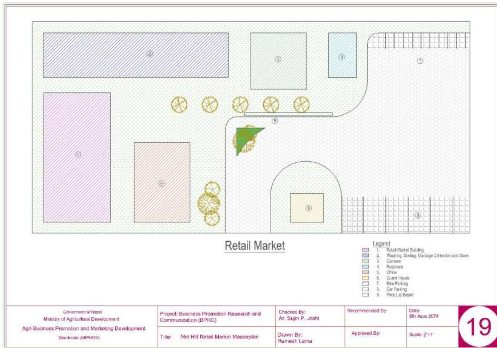
Figure 5.19: Standard design of retail market plan (Mid hill)
