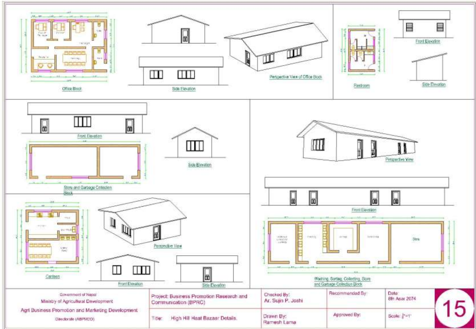
Figure 5.15: Standard design of haat bazaar detail (High hill)
