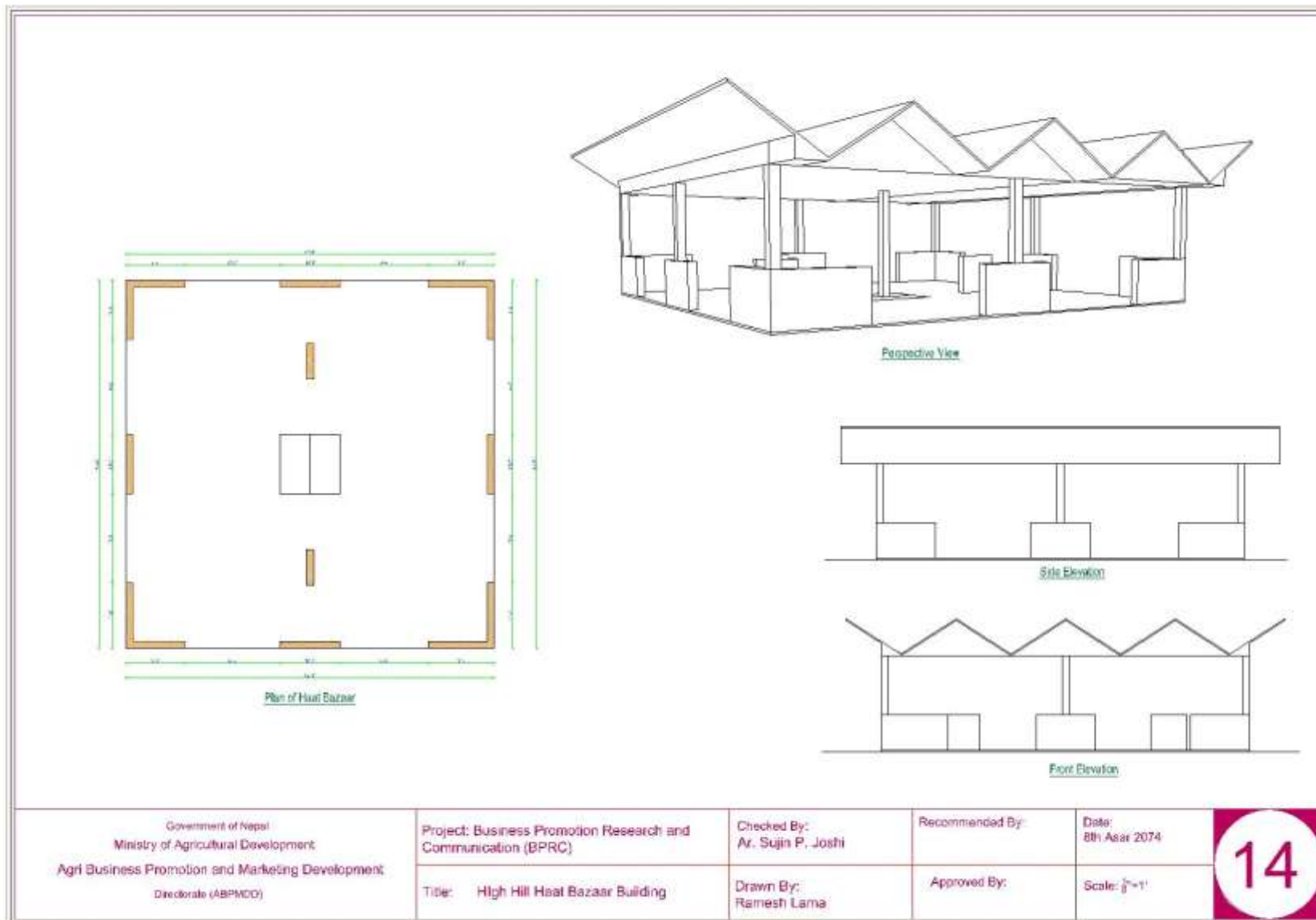
Figure 5.14: Standard design of haat bazaar building (High hill)
