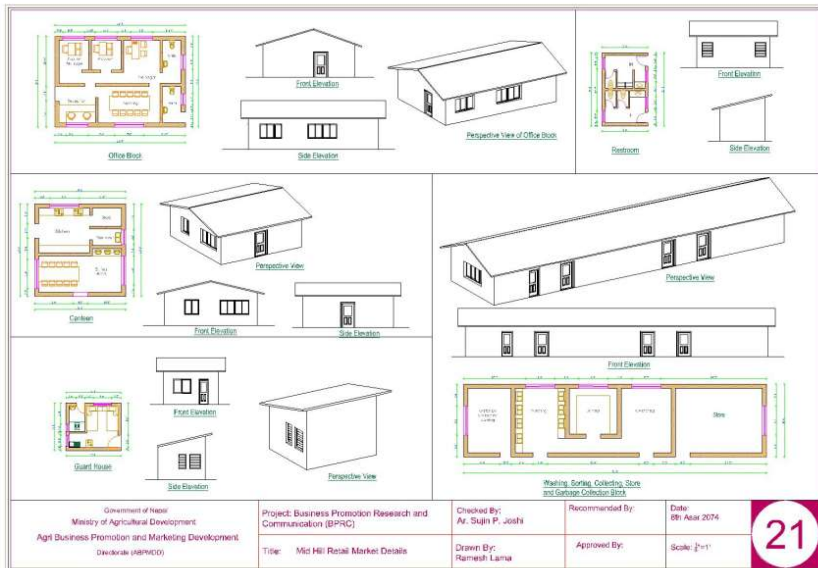
Figure 5.21: Standard design of retail market detail (Mid hill)
