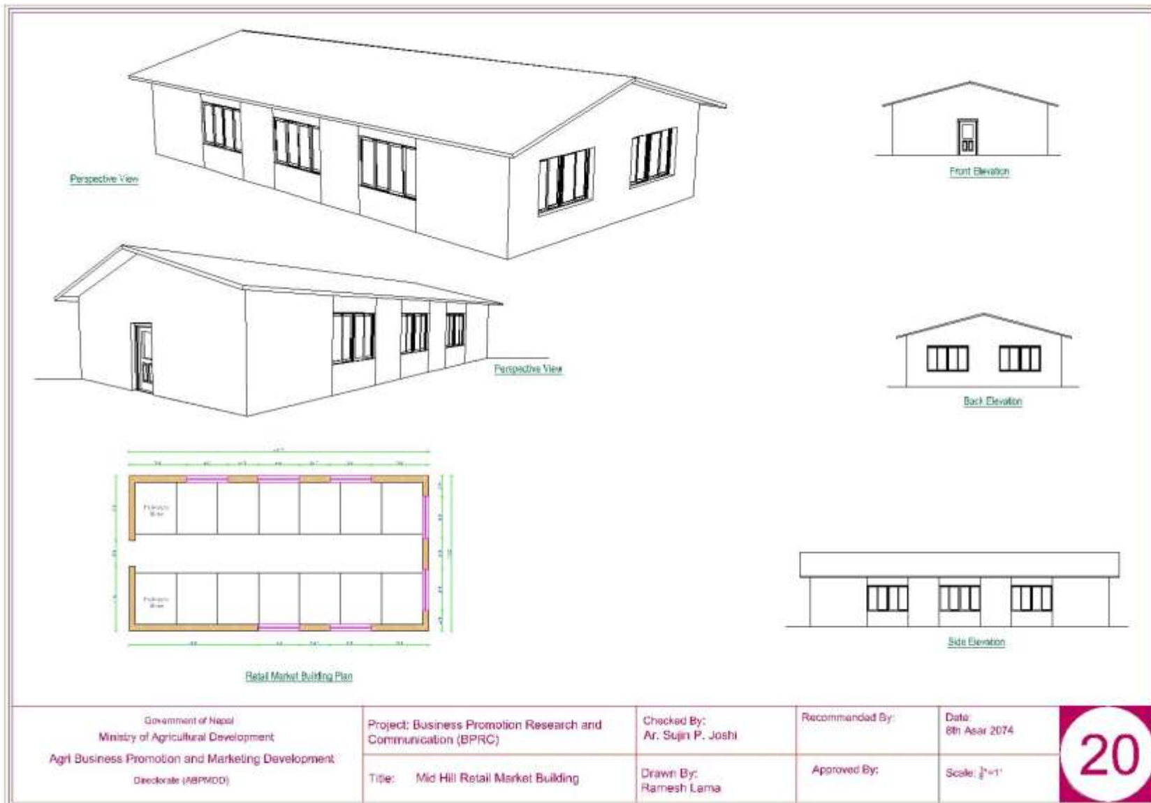
Figure 5.20: Standard design of retail market building (Mid hill)
