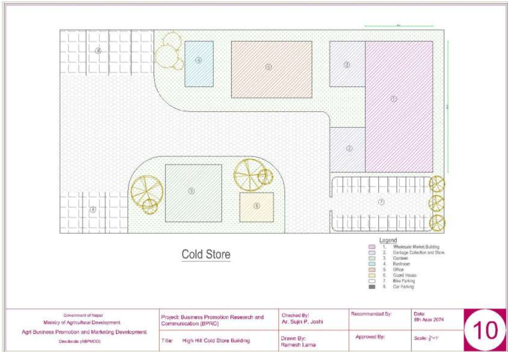
Figure 5.10: Standard design of cold storage plan (High hill)
