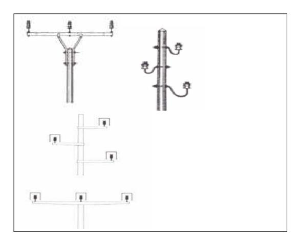
Figure 6-2: Power poles with upright insulators
