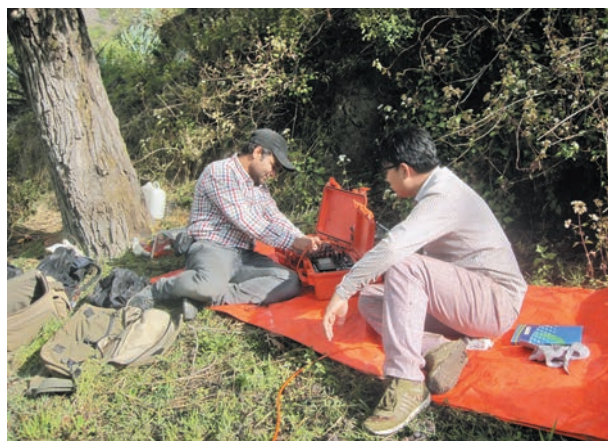
Data acquisition works for ERT Survey.
