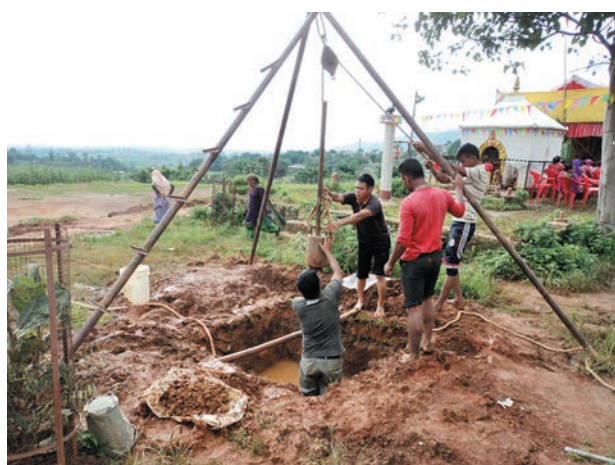
Test pitting SPT at site
