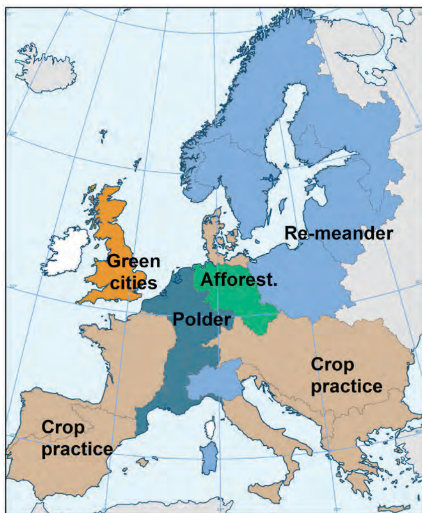
Figure 4.4 Most effective regional NBS measures to reduce flood peaks for a 20-year flood
