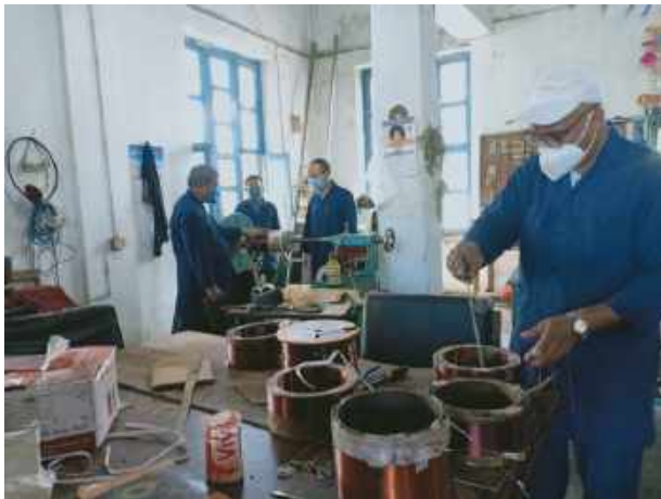
Maintenance of burnt transformers at Transformer Workshop at Pokhara
