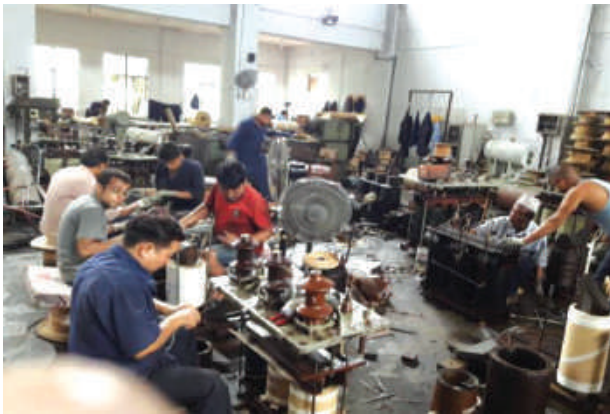
Maintenance of Distribution Transformer
