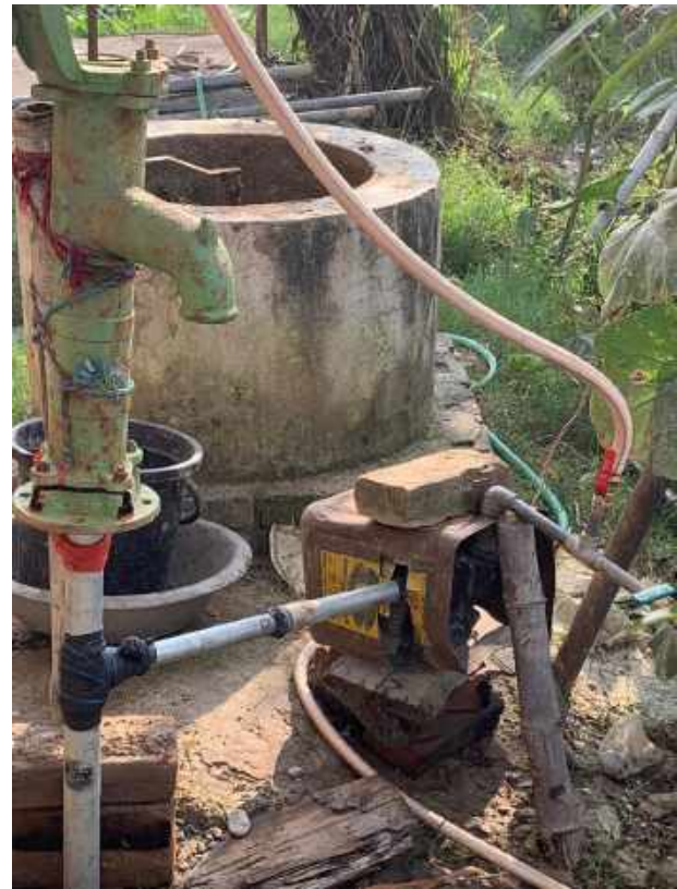
Water pump operating with direct hooking found in Kalaiya DCS
