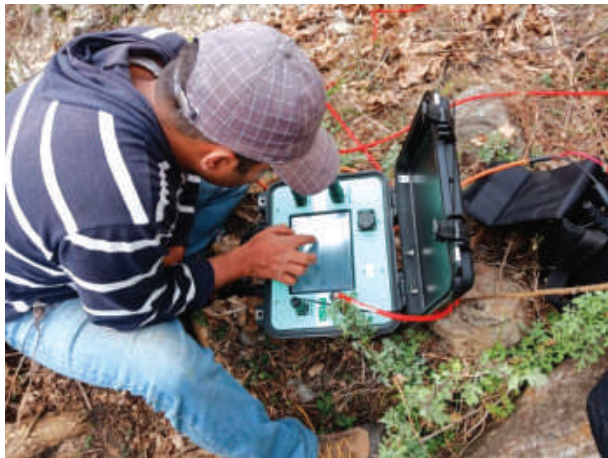
Seismic Refraction survey at Upper Arun HEP
