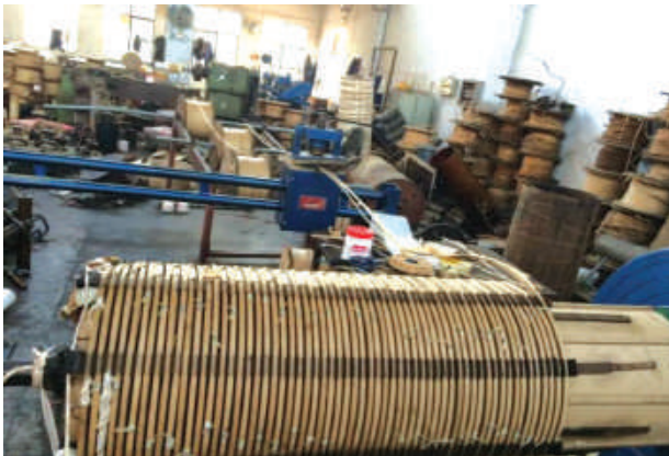
Winding of Power Transformer
