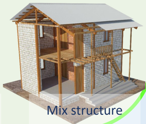
Frame structure + infill wall
